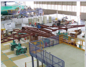
737 - WBJ Unit #4 - Wing/Body Join Tool
