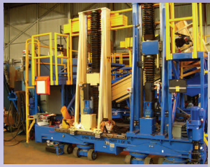
777—MLG Main Landing Gear Loader
